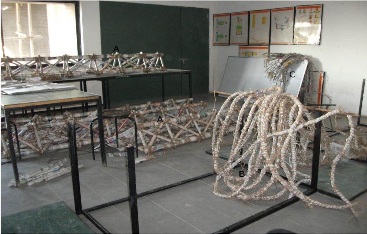
**Fig.-4** A) Piers with bracings; B) Supporting cables; C) Bracings
